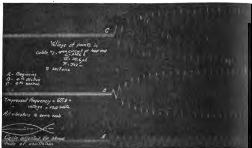
FIG. 83.—Here the artificial antenna was forced to vibrate at three times its fundamental frequency; it will now be noted that the voltages at B and C are in opposite phase in the steady state. From the film it can be seen that the original pulse arrives at C one-half a cycle after passing point B.
